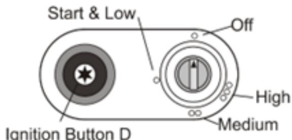
Note: when lighting a new heater for the first time, it might be necessary to hold the control knob down for longer time in order to allow gas to flow to the pilot.
