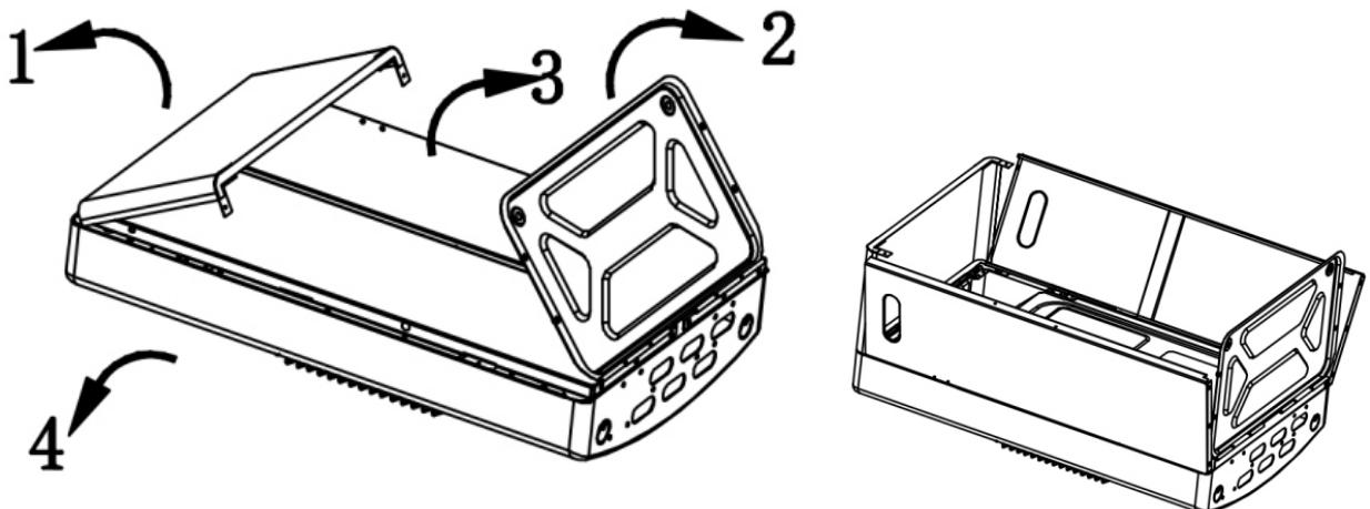
② SECURE THE BEND BACK PLATE WITH FOUR M4 CREWS AND INSTALL THE CASTERS
